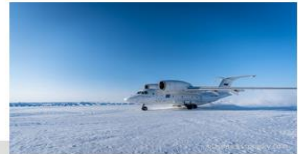
Arctic landing. h=3 m, C_p=25 m/s, Aircraft speed \sim 50 m/s
